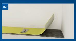
Align the sheet, attach and lay the DURABASE CI-H mat without creases (butt joint installation). Attention: Expansion joints must be taken into account every 40m².
