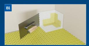
Seal the corners with corner tape and waterproof adhesive ( such as the DURAL DURABASE ET-S internal corners and DURAL CLASSIC FLEX waterproof adhesive ). Please note that the cables must be installed before installing the sealing components.
